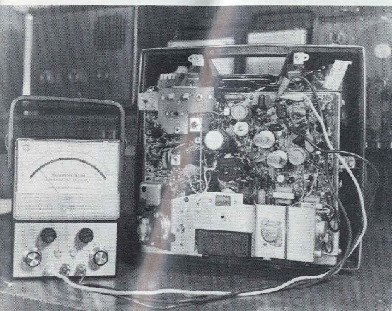
Figure 3: In-circuit beta readings may be lower than out-of-circuit readings for the same transistor.
