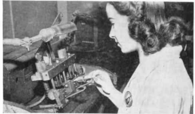
A curtain of light, reflecting across the front of the machine and returned to the Phototube by means of two mirrors, automatically—if interrupted—locks the controls of the machine in safe "off" position. The Magic Brain of every electronic device is a tube . . . and RCA is the fountain head of modern tube development.
