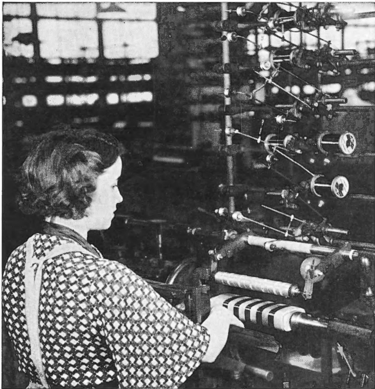
Winding five coils at once helps to reduce the cost of high quality RCA Universal Transformers. Automatic machinery is used to insure precision windings.
