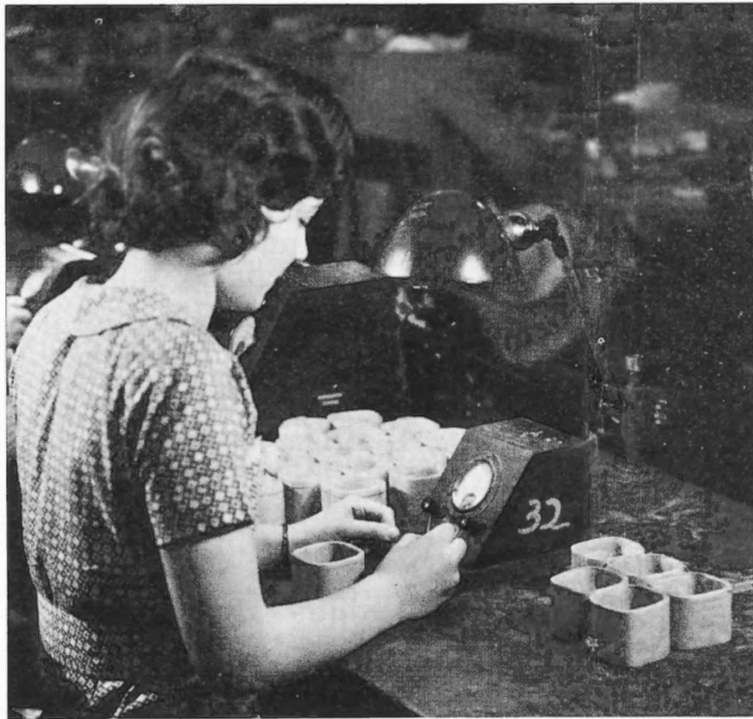
Testing at every stage of manufacture assures perfect products. The illustration shows continuity testing of the plate windings of RCA Universal Transformers.
