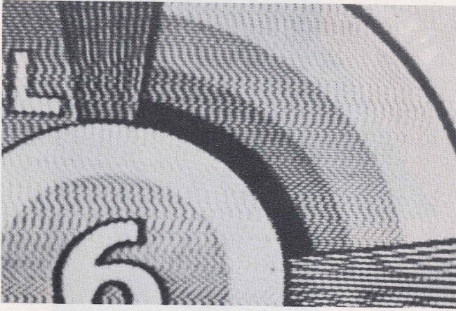
Fig. 3. Third example of interference produced by a harmonic of the sound-if signal falling in a TV channel. In this case, the beat between the harmonic and the rf picture carrier is a high frequency. If a harmonic of the 4.5-Mc sound-if signal causes interference in an intercarrier receiver, the beat frequency is not altered by adjustment of the receiver tuning control.
