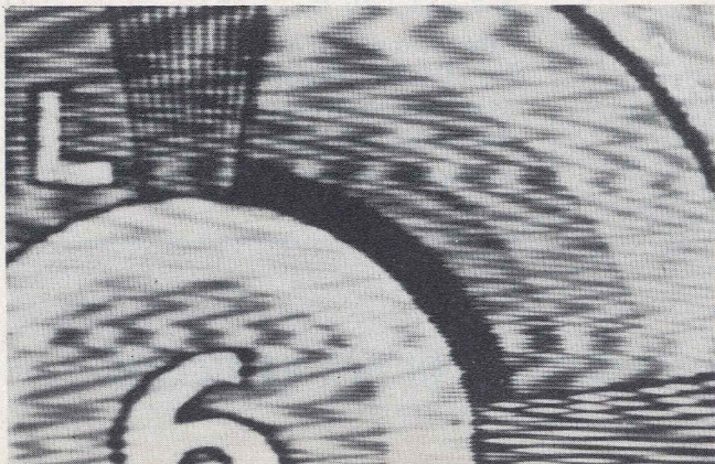
Fig. 1. An example of interference produced by a harmonic of the sound-if signal falling in the rf band. The harmonic energy was deliberately coupled from the output of the sound-if amplifier into the rf-input circuit to produce this interference. In this receiver, the sound if is 21.25 Mc and the fourth harmonic is 85 Mc, which falls in channel 6. In receivers having a separate sound channel, the beat pattern changes with adjustment of the receiver tuning control.
