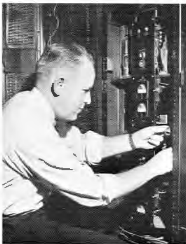
Theatre Service Engineer J. J. Zoltowski changes a tube in a Music Hall amplifier.
