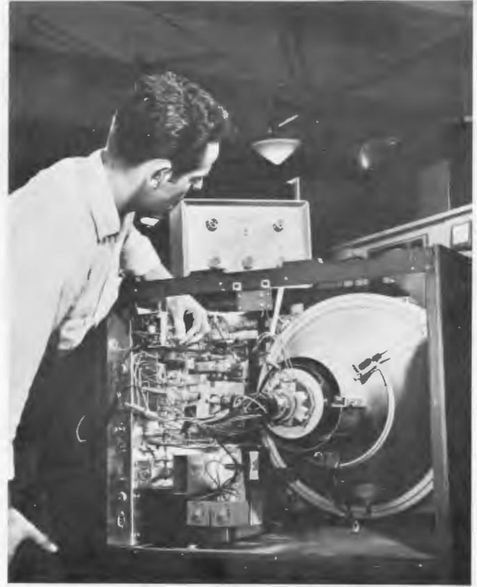
Television and General Electronics Course student uses a Crosshatch Generator to adjust a color set.
