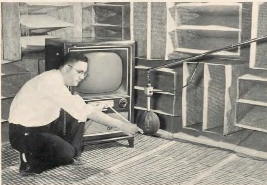
Acoustics Engineer R. L. Libbey (TV Advanced Development), prepares to measure the sound performance of a television set in one of RCA's echo free chambers.
