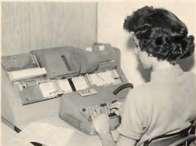
An integrated IBM facility processes large amounts of field performance data on the FPS-16, Data Link and other programs. Above, IBM operator transcribes field reports to punched IBM cards.
