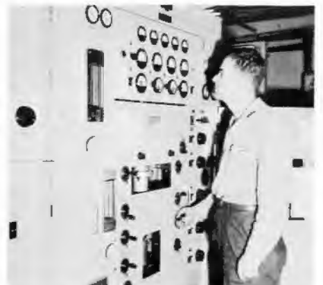
RCA Service Company Government Service field engineer installs equipment. Below, Ralph Bradburn, Iceland Area Supervisor, tunes AN/FRC-39 Tropospheric Scatter Communications Transmitter
