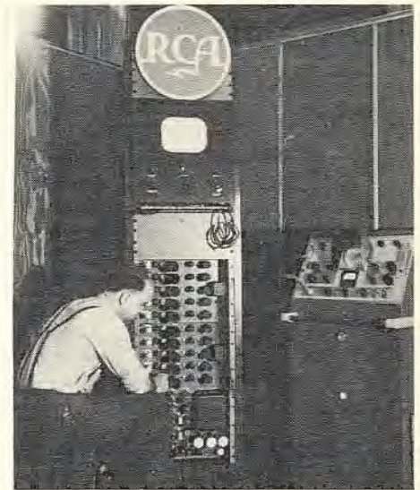
Engineers of the Service Company's television demonstration group were called on months in advance to design and build special equipment which made the display possible. A part of this is seen in the accompanying photo. Don Beck of the demonstration group is making final adjustments on the special TV control and distribution rack used to provide picture and sound signals to the receivers. A high-frequency cathode ray oscilloscope is seen at Don's right.
