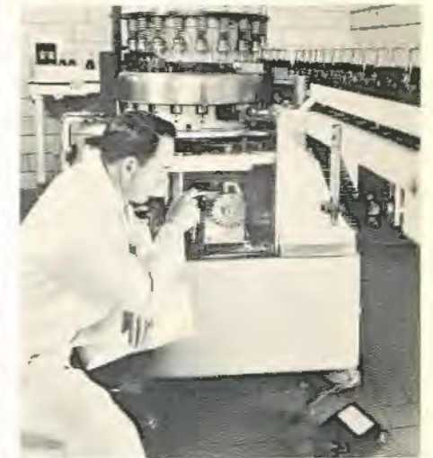
Photo above shows Ken Hallister checking adjustments of timing switches on the Beverage Inspection Machine at Coca-Cola's Camden Bottling Plant.
