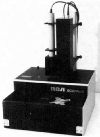
Fig. 4—Mechanical unit of scanner, red version with HeNe laser (6328 Å).
