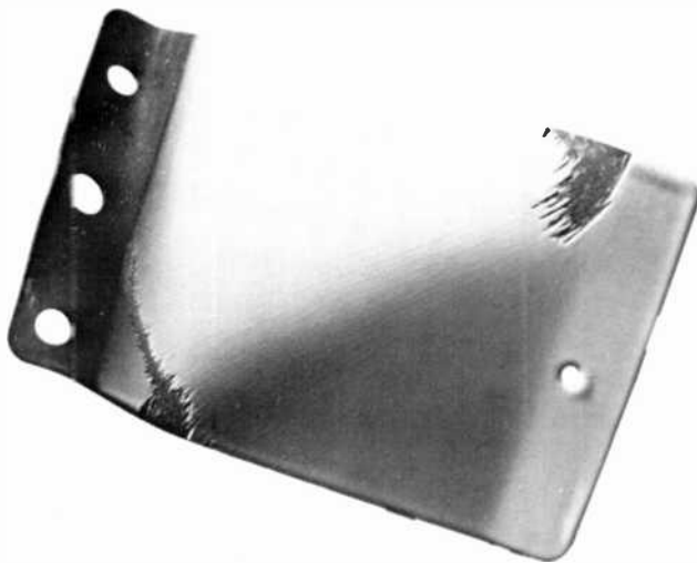
Fig. 19—Torsion tested sample of RCA porcelain.
