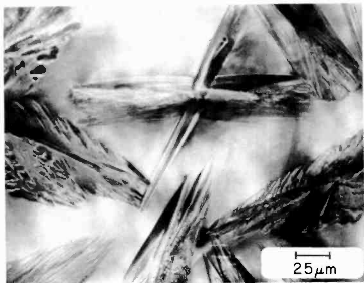
Fig. 6—Crystal growth from the melt—initial stage.
