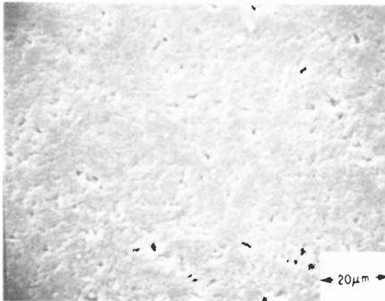
Fig. 1—Scanning electron micrograph of surface of RCA porcelain-coated steel substrate.
