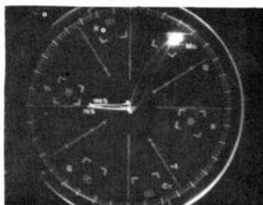
C) Magenta Field Vector with Static C.B. Interference (1%)
