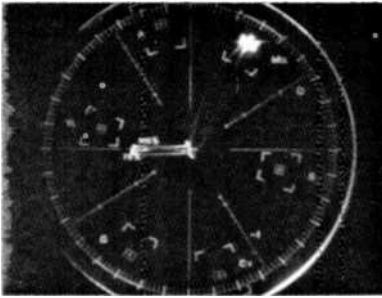
(A) Two main vectors with locus of points, CW interference and AM in the interfering channel
