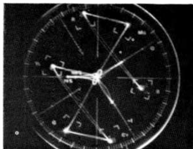
B) EIA Color Bars Vectors without Interference
