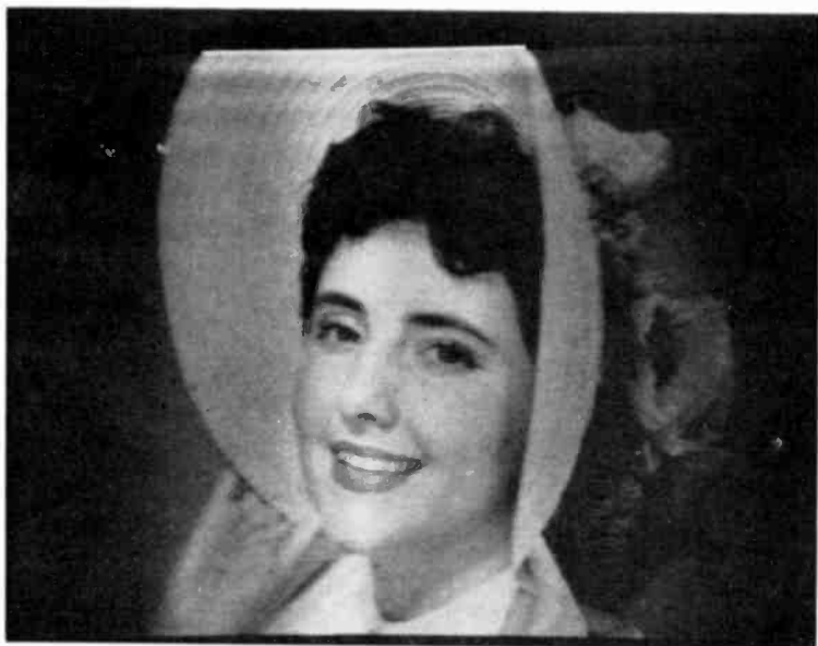
Fig. 7—"Typical" test subject displayed by the laser scanner, using a galvanometer vertical deflector.
