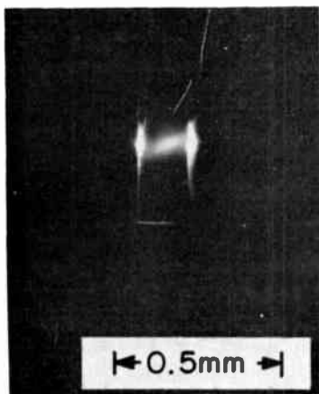
Fig. 3—Photomicrograph of one CdS crystal emitting laser light at corners.
