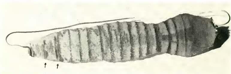
Fig. 5—Rate-grown crystal which comprises only two p-type layers near the seed end of the crystal (arrows). The dark bands are the highly doped regions which have etched more than the rest of the crystal.
