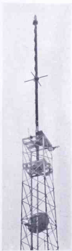
Fig. 26—67.25-megacycle turnstile antenna used in UHF-VHF comparison survey mounted at radiation center of UHF antenna.
