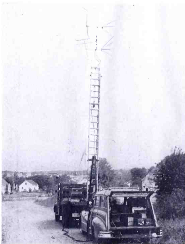
Fig. 27 — Mobile equipment used in UHF-VHF comparison survey.
