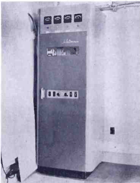
Fig. 25 — 67.25-megacycle transmitter used in UHF-VHF comparison survey.
