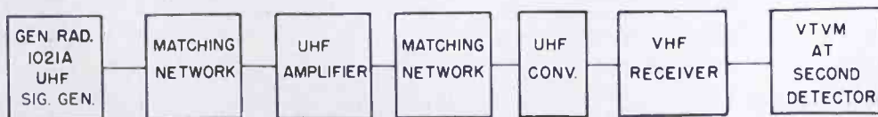
Fig. 16—Block diagram of noise-factor measuring equipment.
