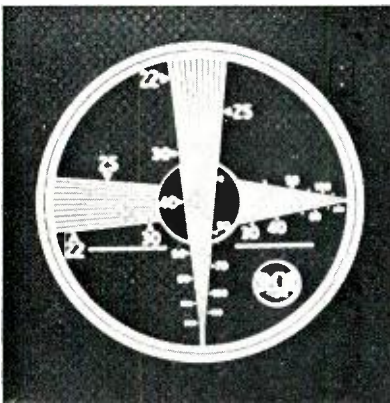
Fig. 94—Photograph of test pattern obtained by an optical aperture with characteristics given by curve 1, Figure 93.
