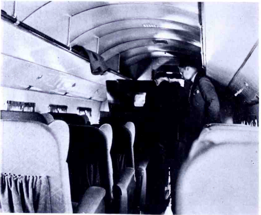
Fig. 2—The television receiver installed in the forward part of the passenger compartment.
