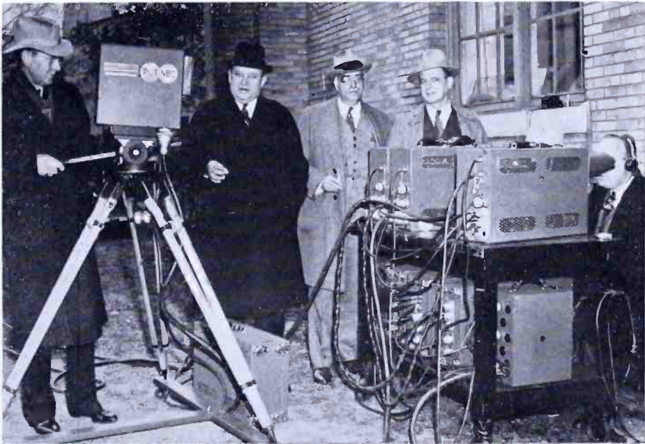
Fig. 1—FCC members see new RCA television field equipment, (left to right) James Lawrence Fly, Chairman of the FCC, handling the television camera; Commissioners Thad H. Brown, Norman S. Case, and T. A. M. Craven. The complete unit is not only more efficient than, but also approximately one-tenth the weight and one-sixth the cost of the only other unit ever designed in this country for the same purpose.
