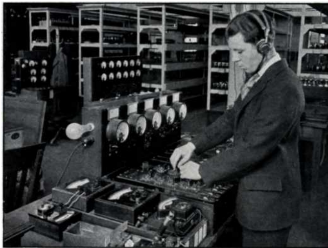
Testing RCA Radiotrons for amplification factor, plate resistance and other characteristics
