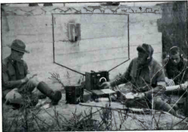
Signal Corps soldiers operating the SCR-77B field radio set, which is used for communication between front line battalions and their regimental headquarters
