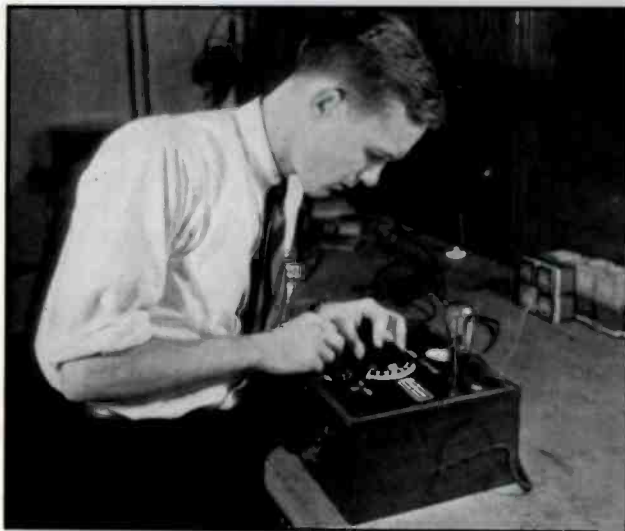
The oscillator can be used as a wavemeter once it is calibrated
