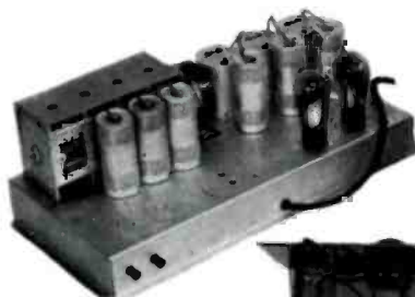
Above—modern Silver-Marshall chassis exemplifying simplicity and shielding
