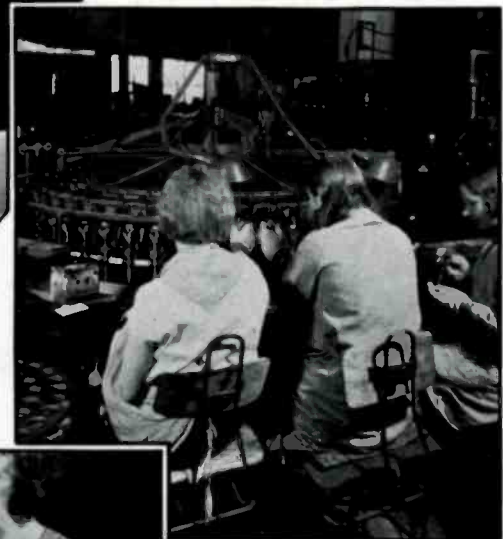
This carefully supervised ma- chine cements the bases to the bulbs
