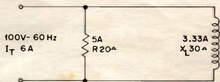
Figure 4—Inductive Reactance
