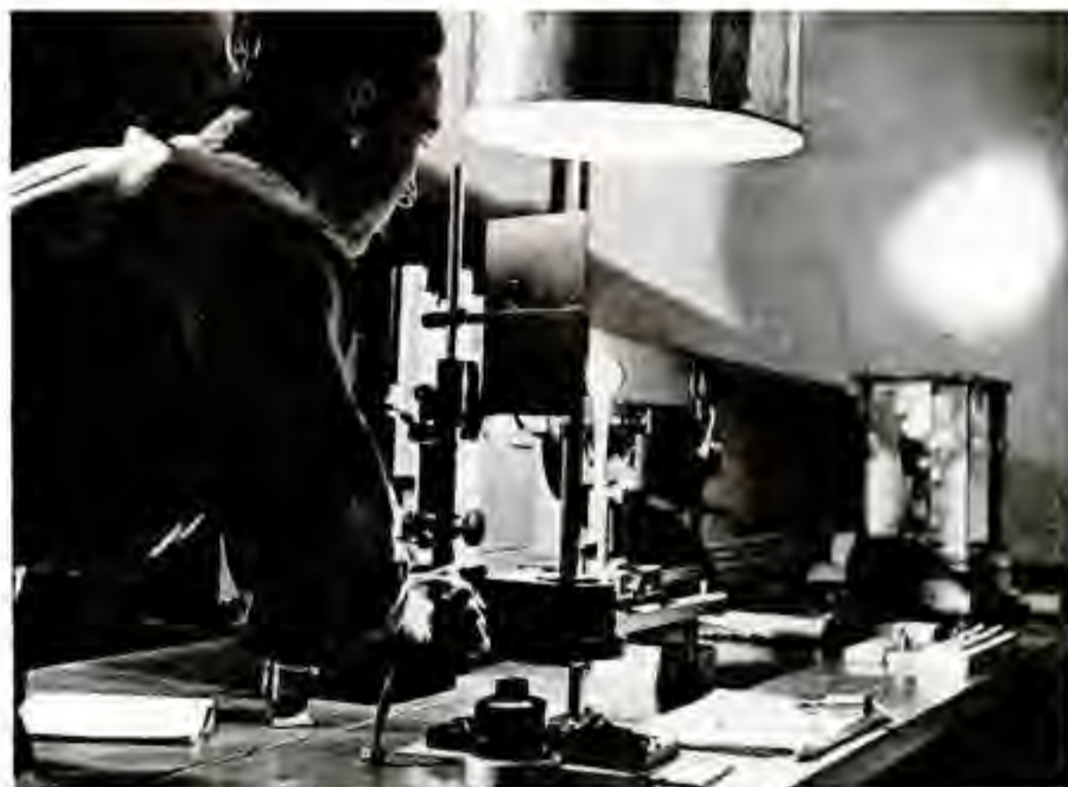
Tube materials must be pure —This spectrograph is used to test purity of materials used in making RCA Radio Tubes. Volatilized in a carbon arc the material produces a spectrum which is photographed with aid of a quartz prism. The quantity of each element present is indicated in the resulting picture.
