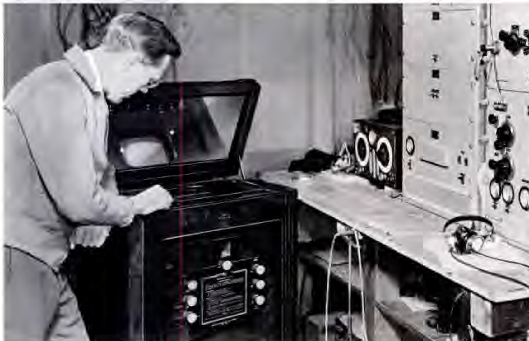
Another radio frontier. Recent television tests suggest that its satisfactory broadcasting may be limited to a radius of about 40 miles. But RCA engineers, always impatient with apparent limitations, are determined to investigate this matter further. They built the super-sensitive receiver shown above. This was connected with a special antenna at Riverhead, Long Island. The sound signals from television programs in London are clearly heard on some occasions. So far, no pictures have been caught. What these experiments may mean in the future of television no one can say as yet, but they well illustrate the constant endeavor of RCA engineers to push the frontier of radio knowledge farther forward.
