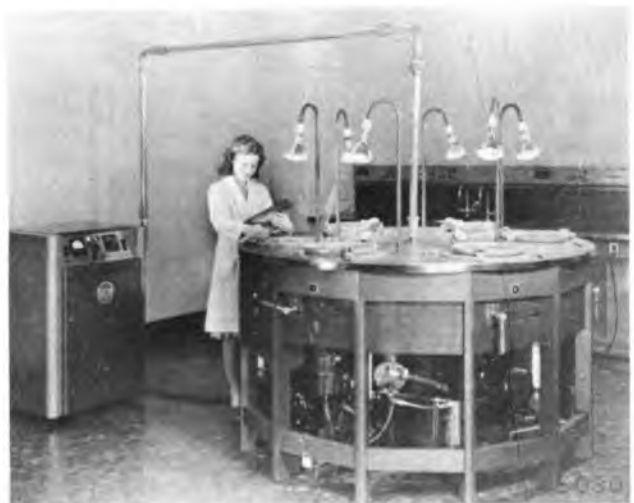
Method of Handling Ampoules in Drying Chamber on Table Containing Six such Chambers is Illustrated by Miss Veronica Moran. Infra-red Lamps Prevent Condensation on Cold Lids of Vacuum Chambers.
