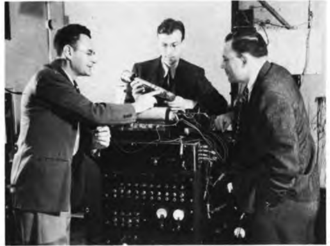
Doctors A. Rose, P. K. Weimer, and H. B. Law Discussing the Image Orthicon
