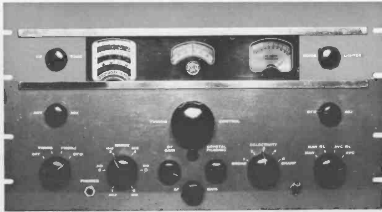
Figure 1: Front panel of the RCA-CR-91 general-purpose communications receiver. The AGC switch (extreme right) was subsequently modified to include "SSB" in a fifth position.
