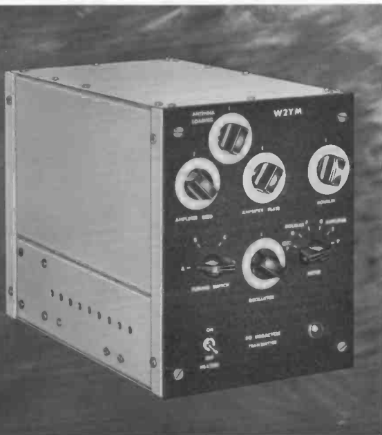
Front view of W2YM's 120-watt 50-megacycle transmitter. [Note the air-intake holes on the side of the blower (or bottom) chassis. They each measure 3/8 inch in diameter.]
