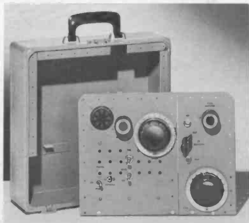
Four brackets made of 3/4-inch aluminum angle are utilized. One supports the power-supply "deck." The others, mounted on three sides of a portable typewriter case, support the front panels of W2QEX's 40-meter cw station.
