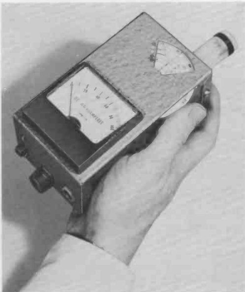
The transistORIZED grid-dip meter described in this article measures only 2\frac{1}{4} by 3 by 5\frac{1}{4} inches. It can be held and operated with one hand.
