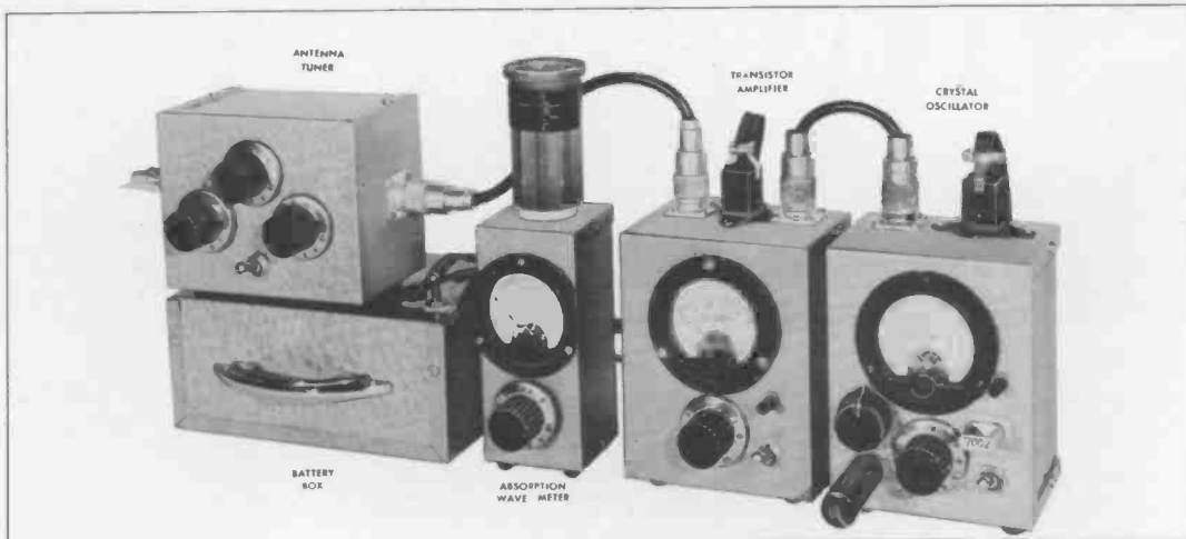
Complete transistor rig. Maximum input to the final amplifier: 216 Mw.
