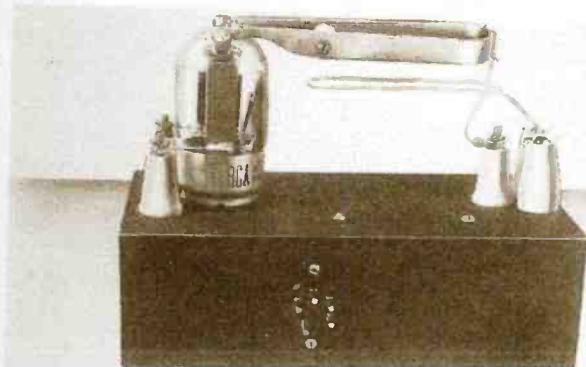
Top view of the transmitter. A little bit of copper and a few ceramic insulators put the 815 to work.
