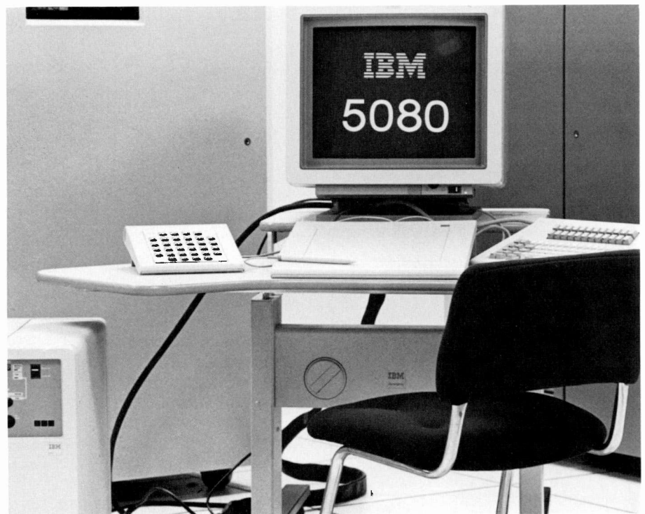
Fig. 2. IBM 5080 graphics workstation. The workstation consists of a 5081 CRT display, a typewriter keyboard (left), a cursor tablet (center), a lighted function key pad (right), and a 5085 graphics processor (right, on the floor).
