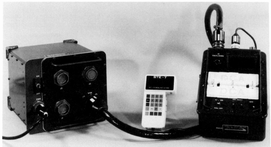
Fig. 1. Simplified test equipment for the Abrams M1 tank and the Bradley Fighting Vehicle System.
