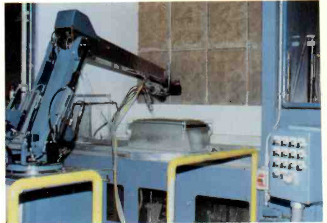
Spray paint robot used in television manufacture at Indianapolis, Indiana
