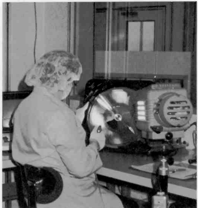
Fig. 6. Inspection station. The parts are inspected for defects using a grazing incidence light inspection, which highlights microscopic defects.
