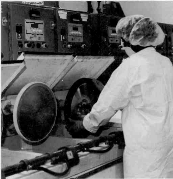
Fig. 5. Nickel plating bath. The parent part is loaded onto the nickel plating tank for deposition of an electroformed daughter part. The daughter will be the reverse image of the parent.
