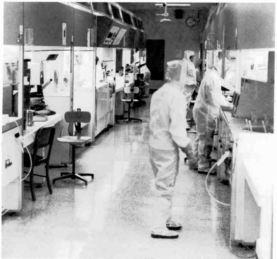
The etch and inspect line. Chemical etch sinks and rinse tanks are on the right. Binocular microscopes on the left are under laminar flow to combat particulate contamination.
