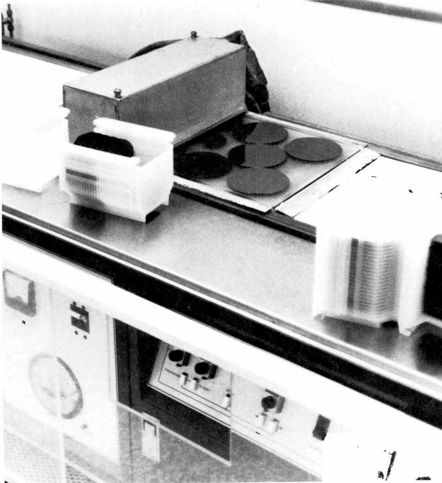
Deposition of a protective layer of silicon dioxide on the almost-finished wafer permits later handling of the individual circuit in the assembly process, and imparts desired electrical or reliability characteristics.
