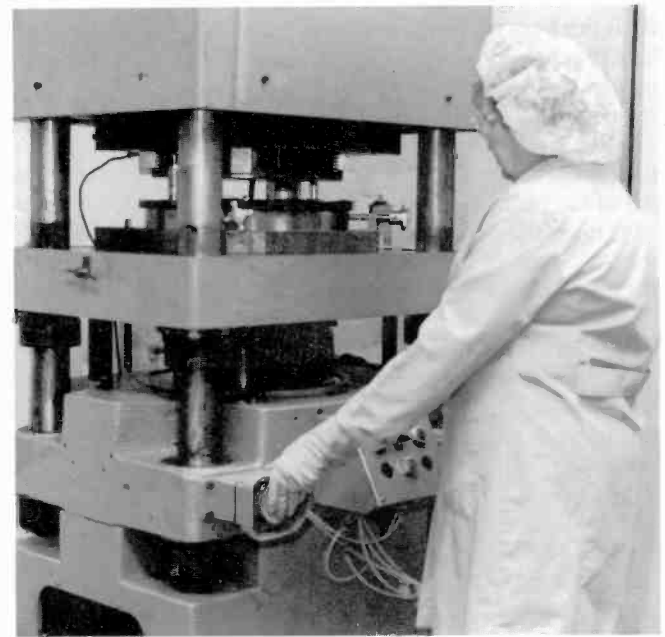
Fig. 10. Coining die. The mechanical profile of the inner and outer edges of the stamper is formed in a coining operation. The forming allows a match between the stamper and the press-mold geometries.
