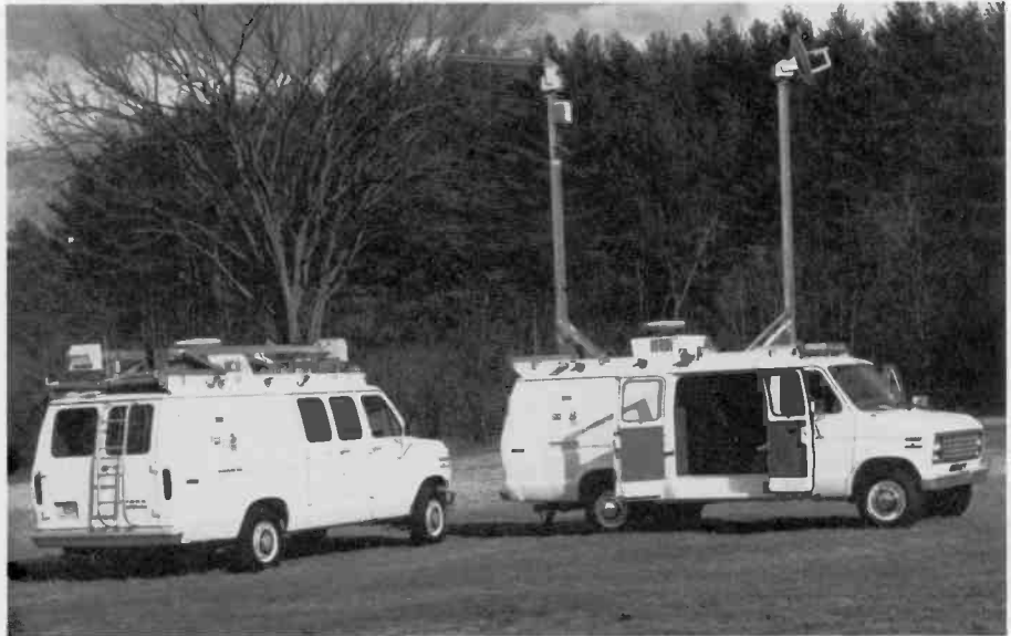
Fig. 5. WNBC-TV mobile microwave vans. Fold-over masts are shown extended and retracted.
