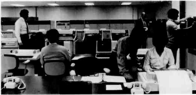
Overview of the Naval System Department's Program Generation, Analysis and Data Reduction Center, showing three DECSYSTEM-2060s behind the disk drives. The two VAX 11/782s are behind the DECSYSTEM-2060s.
