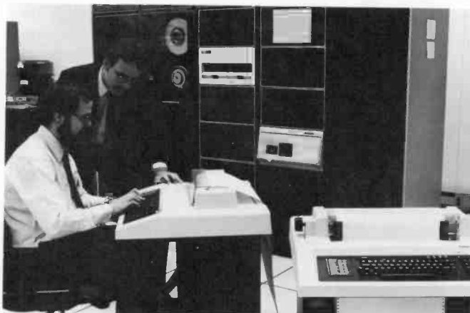
A direct-access console is provided for each computer in the SDF network to allow system debugging.
