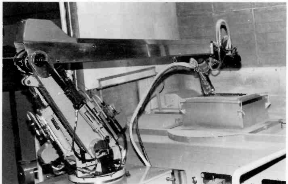
Fig. 4b. The robotic spray-paint system.
