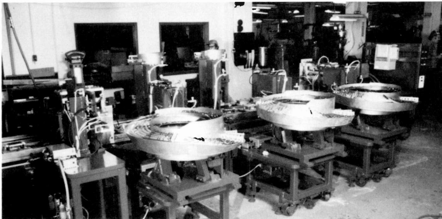
Fig. 6b. This view of the switch-assembly machine shows the actual system under construction. In the foreground are the vibratory feeders for switch components.
