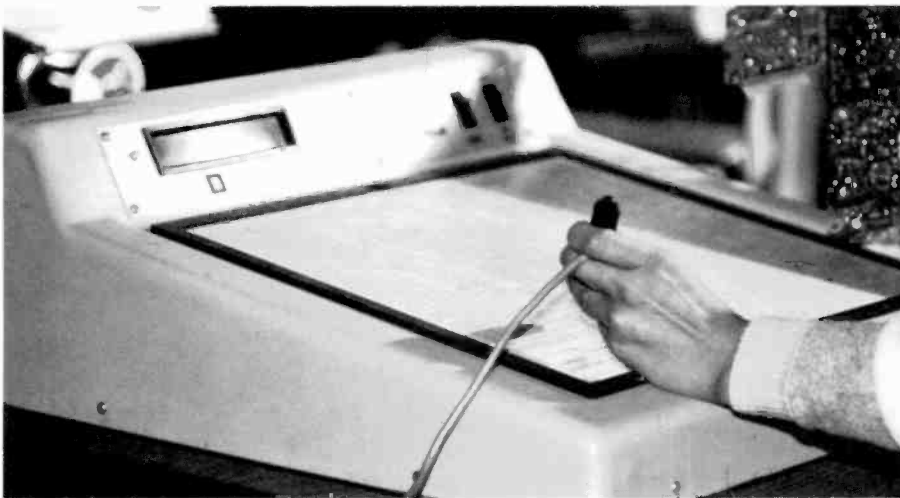
Fig. 3. The FRED terminal. This custom-designed terminal is one of several located on each manufacturing line. It is used to transmit chassis serial numbers, repair codes, and part legends to the data-collection computer. Its digitizing tablet is used to translate line data into defect and repair codes.
