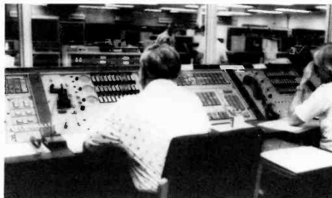
MTP System Controllers direct operations at the Central Computer Complex, and supervise the data interface with display systems and worldwide tracking sensors.
