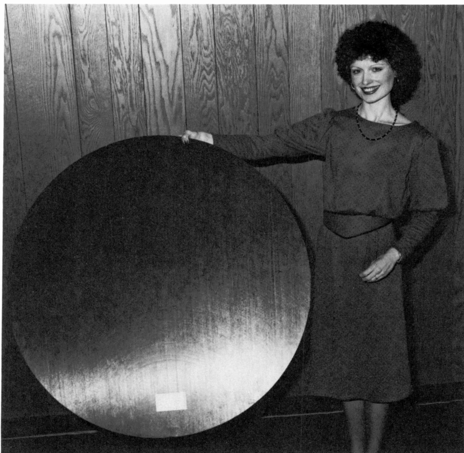
Fig. 4. Solid single-shell reflectors offer extreme dimensional stabilities (less than 0.003-inch rms distortions) under mission thermal environments.
