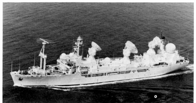
Fig. 8. MTP people on board Range Instrumentation Ships use radar, telemetry and photographic systems to track missile and space-vehicle components, such as Space Shuttle solid rocket boosters, which impact in the ocean.
