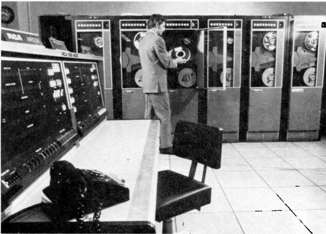
Fig. 4 Computerized message switching system for leased-channel subscribers is called AIRCON. System handles high-speed traffic, giving urgent traffic priority and selecting alternate routes if the original route is interrupted.
