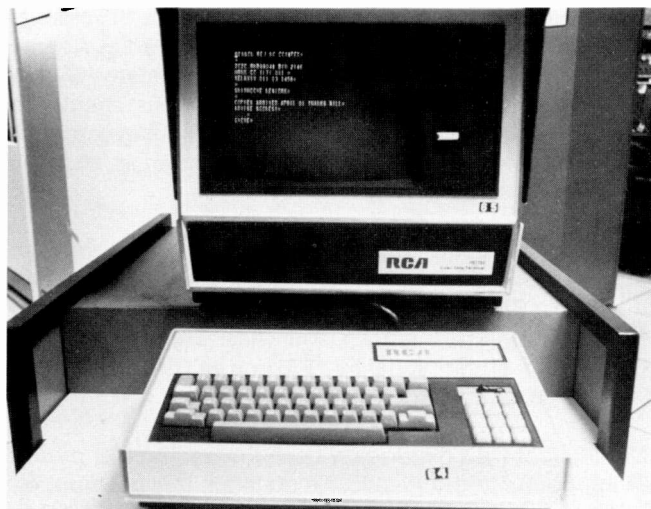
Fig 1 Automatic retrieval computer (ARC) is an example of telegram-facility automation. Telegrams for overseas destinations must fit into a proper international format; the ARC automatically removes messages from the Computer Telegram System (CTS) that are not in the correct format and displays them on this CRT monitor. Operators make needed corrections and then route the telegrams back to the CTS.
