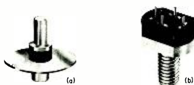
Fig. 2—Photograph of two transistor packages specifically designed for operation at uhf and microwave frequencies: a) coaxial package, b) stripline package.
