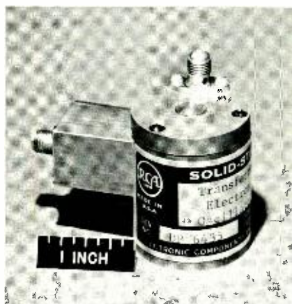
Fig. 9—Photograph of a pulsed 100-watt L-band transferred-electron oscillator.
