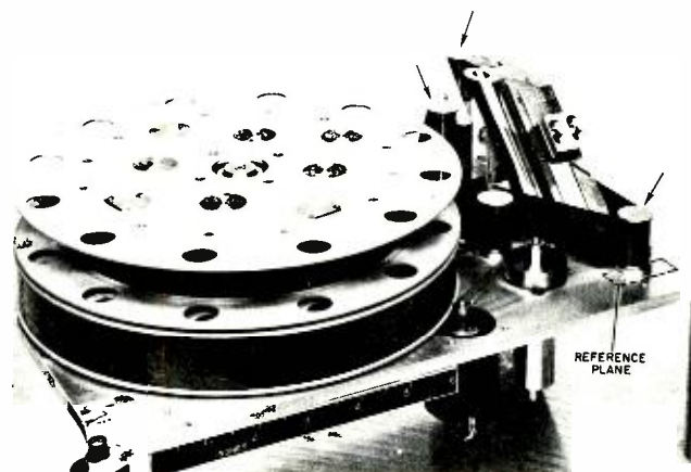
Fig. 1—Magnetic recorder showing tape-guide rollers (arrows).
