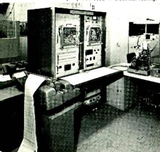
Fig. 2—High-speed automatic test equipment and multiple probe used in electrical testing.
