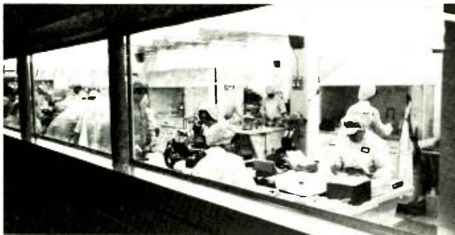
Fig. 3—View through window in Laminar Flow Room showing the Wafer Photolithography Processing Area.
