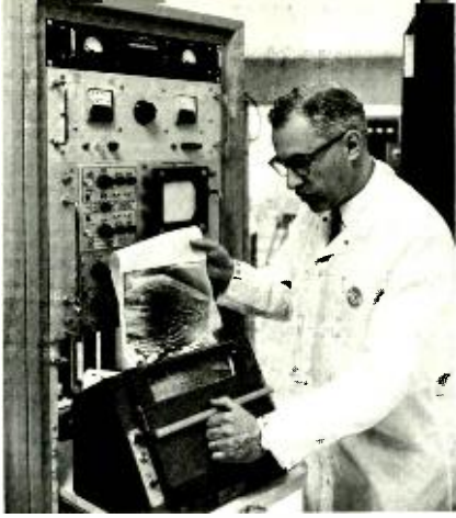
Weather pictures from the RCA APT camera system on the Nimbus II satellite are automatically transmitted to small ground stations where they are reproduced on a facsimile machine as shown. Storage of the weather picture on the APT camera vidicon tube permits transmission to simple ground stations located in any area of the world. The APT system is one of two advanced RCA television systems aboard the experimental Nimbus II satellite.
