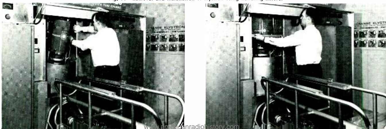
Fig. 11—Removal and installation of klystron using handling fixture.
