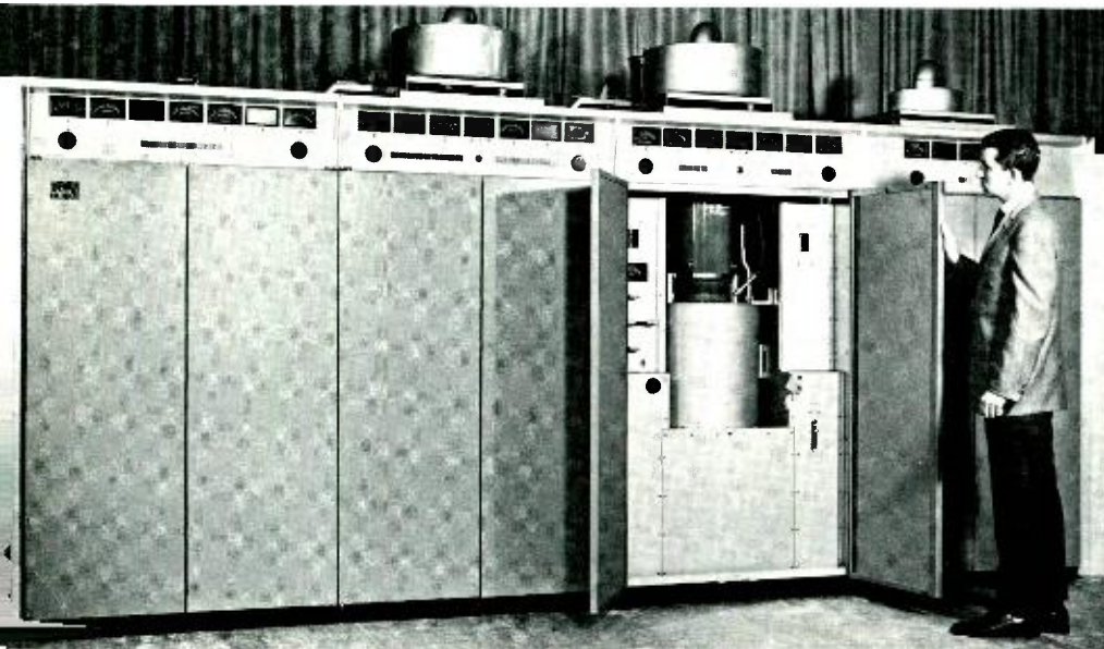
Fig. 1—View of the main RF and control cabinets for the TTU-110A transmitter.
