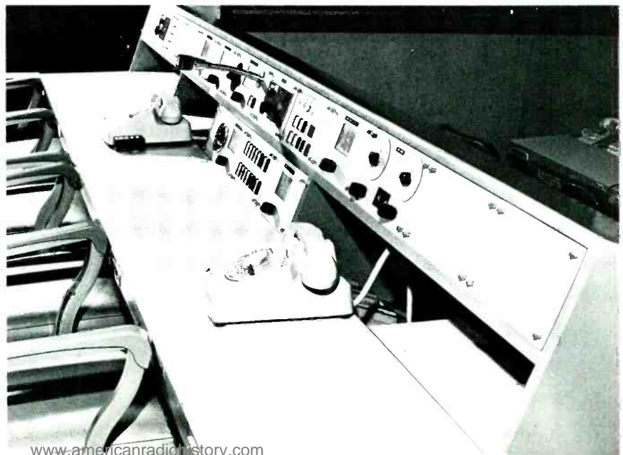
Fig. 8—This "VIP" console contains monitoring, communications, and switching facilities.
