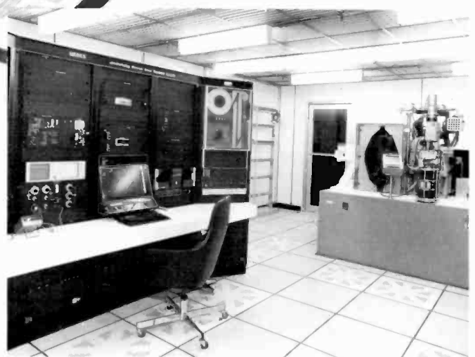
2. Mask generation depends on electron-beam precision exposure. The location of the beam is monitored by an interferometer to 1/32 of a micrometer. For better accuracy, chromium on glass masks is preferred to emulsion on glass masks.
