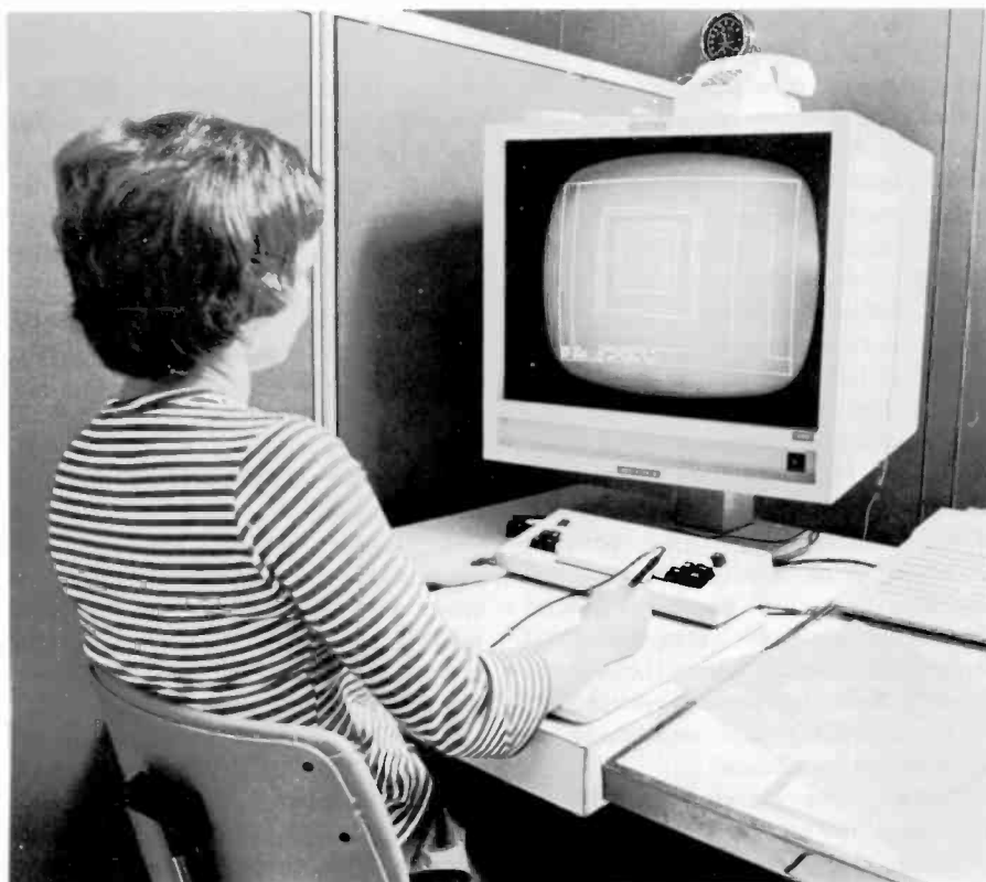
Fig. 6. Using the Applicon interactive graphics system, the operator can easily and quickly make numerous changes to the IC artwork.
