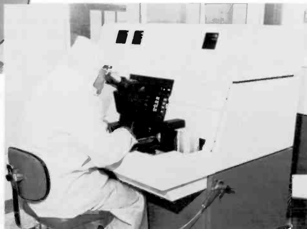
6. Mask defects will print on wafers. If a perfect mask never touches the wafers, better yields can be expected. This Perkin-Elmer aligner uses scanning-projection mirror optics that allow deep-ultraviolet exposures for better resolution.
