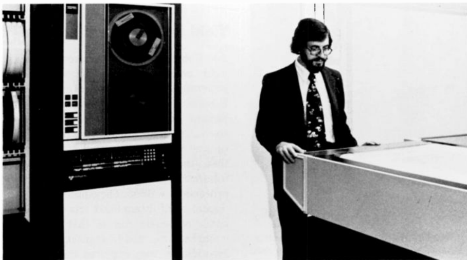
Fig. 5. A 72-inch Versatec Plotter that allows preparation of paper drawings of information on magnetic tape at almost any scale factor in about 8 minutes. This machine is used to checkplot a MEBES tape input before a MEBES is drawn.
