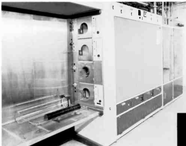
12. Chemical-vapor deposition is used to deposit polysilicon, silicon dioxide, silicon nitride and phosphosilicate glasses. By reducing the pressure, 100 or more wafers can be treated in one cycle. The uniformity of such low-pressure chemical-vapor deposition (LPCVD) systems is much better than that of atmospheric systems. Again, micro-processors control the process.
