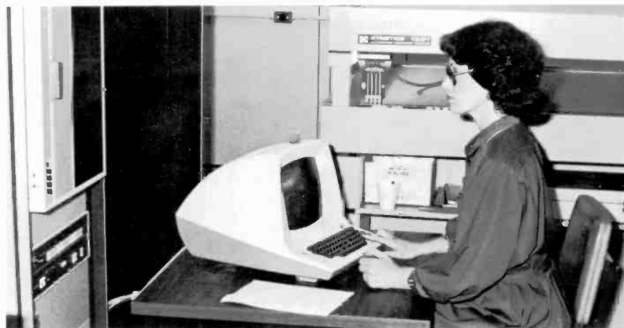
Fig. 7. This electrostatic checkplotter can create a six-foot-square checkplot of a complex IC in less than 10 minutes.
