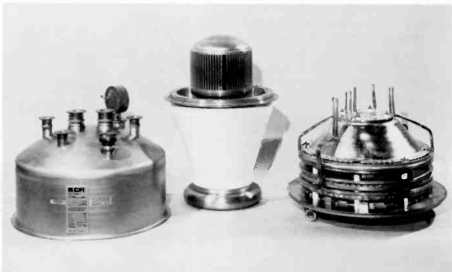
Fig. 3 The three major S94000E assemblies. From left to right: envelope, plate-ceramic insulator and grid-filament.
