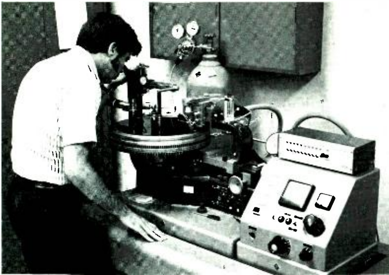
Fig. 1 — Music is transferred from tape to the master disc by means of motional feedback controlled cutter on lathe with variable pitch and depth.
