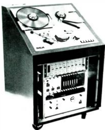
Complete prototype slave unit with the front door removed to show the electronics.
