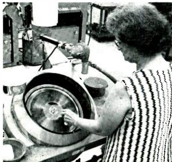
Fig. 5 — Metal mold is polished to remove "horns" produced in master cutting.
