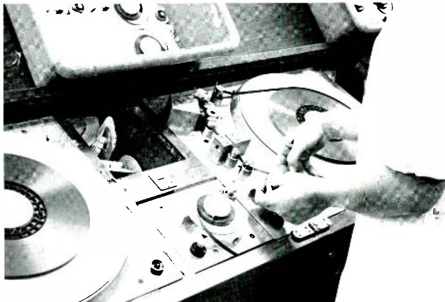
Fig. 3 — Tape breakdown operation separates 7500-ft tape reels into individual programs.
