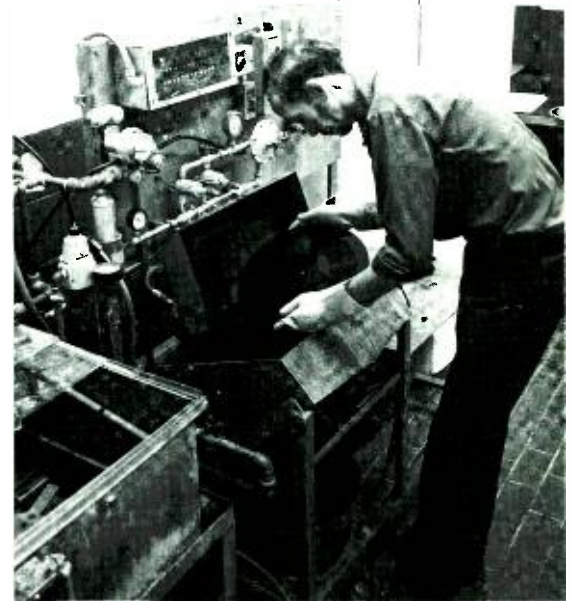
Fig. 2 — Master disc is about to receive silver coating that provides conductivity for further plating.
