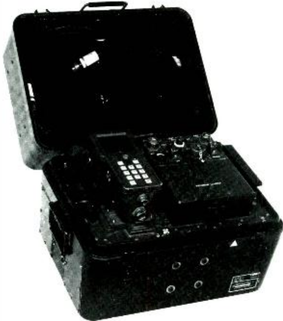
Fig. 1 — Automatic Test Equipment for Internal Combustion Engines (ATE/ICE).
