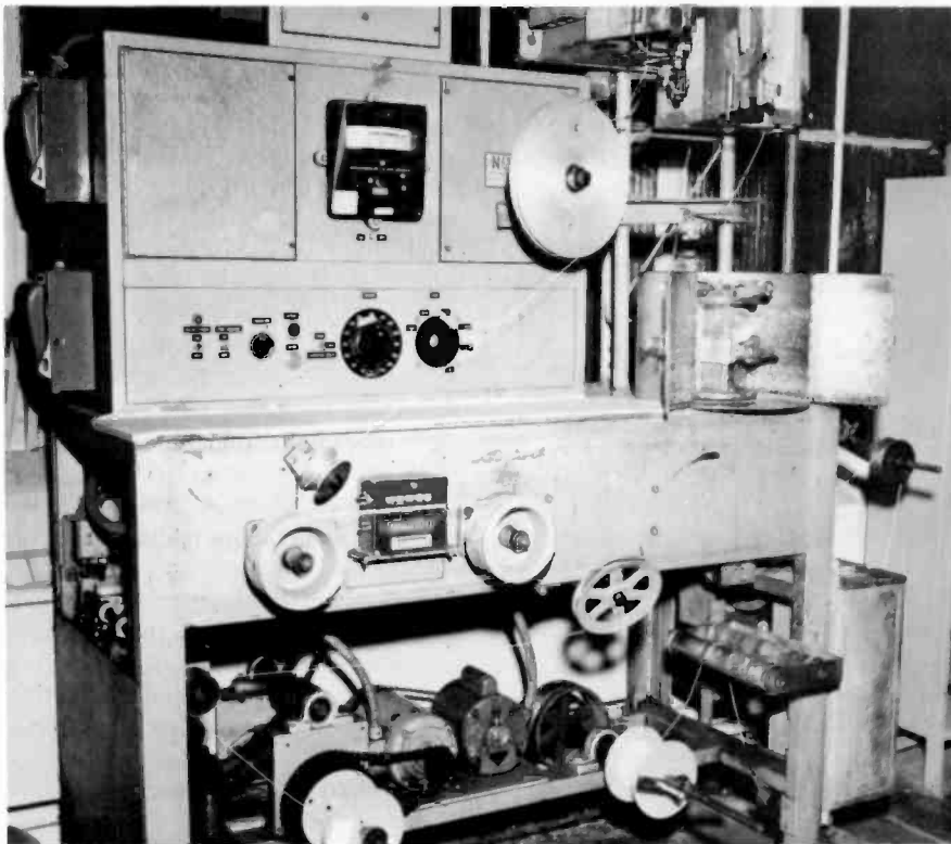
Fig. 3 — Automatic wire color-coding equipment.
