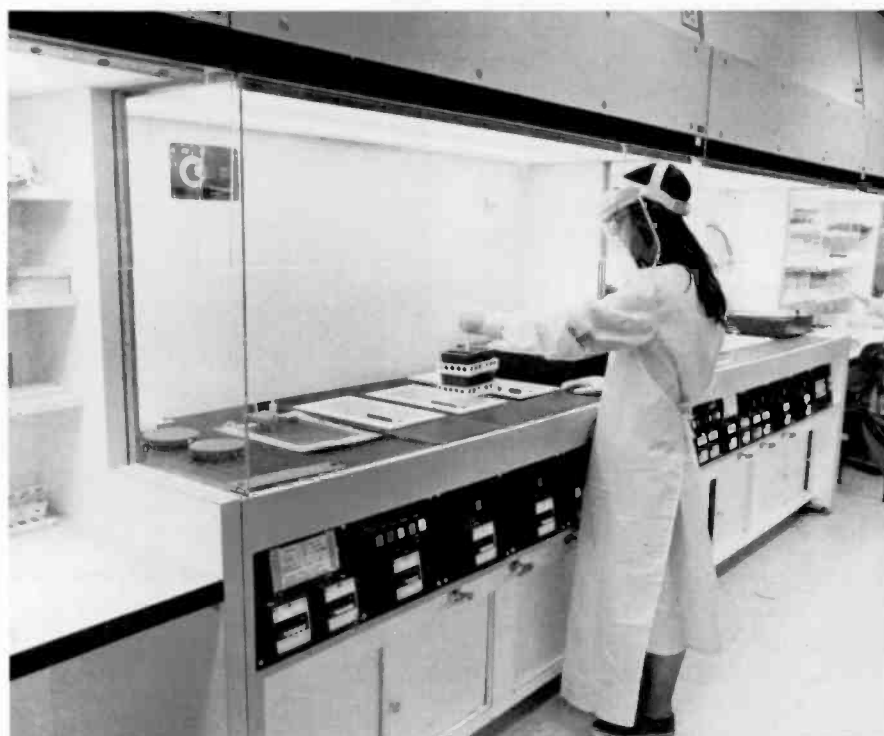
Fig. 3 — Typical DART chemical processing station contains five modular processing units with corresponding front-mounted control panel.
