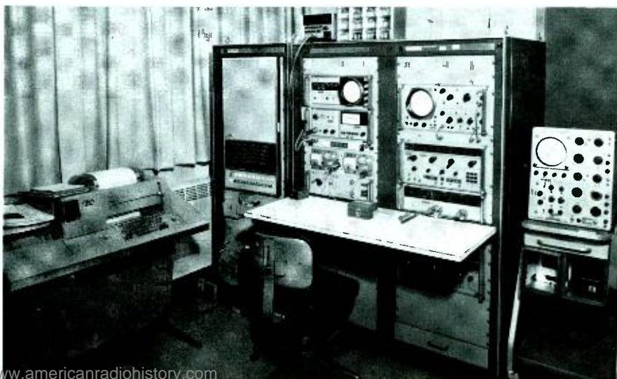
Fig. 6 — Automatic network analyzer (ANA).
