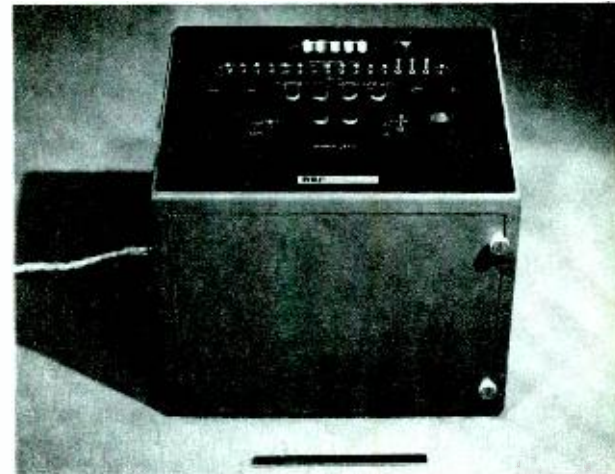
Fig. 11 — The Space Ultrareliable Modular Computer Demonstration Vehicle (SUMC/DV) which was developed for NASA. SUMC/DV is a 16-bit general purpose computer with approximately 35 instructions in its instruction set. Its logic subsystem consists of well over 6,000 logic gates. SUMC/DV was designed, debugged, and delivered in slightly less than one year.
