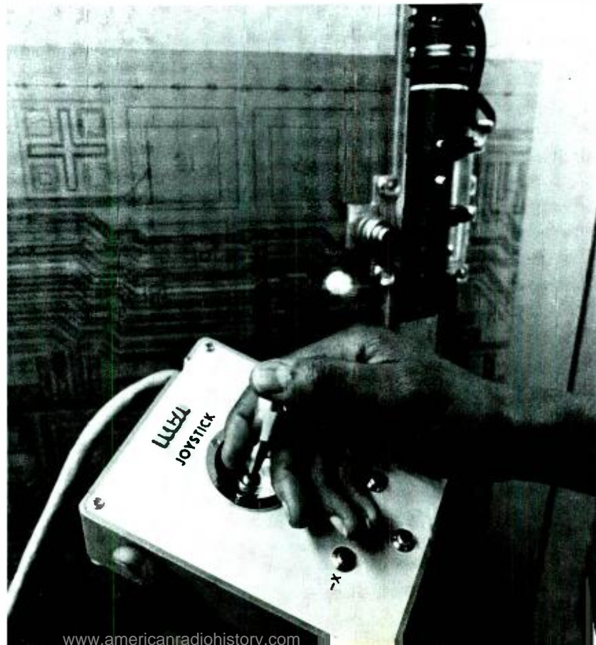
Fig. 4 — Digitizer-plotter system light pointer and joystick.
